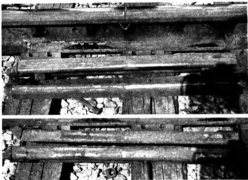
Fig. 10. South Portion Section 5, No Lubrication (Plastic E-plugs both ends)
